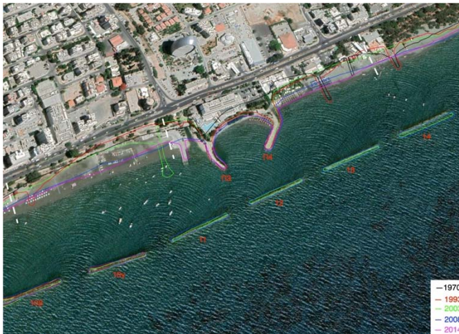
Figure 2. Satellite derived shoreline for Vathia area in Limassol, southern Cyprus with shoreline positions over time indicated with different colors. Transect locations, A, B and C are indicated with white dashed lines (left to right) demonstrating a behaviour of 0.6\pm 0.1 , 0.5\pm 0.2 and 0.2\pm 0.01 m/yr, respectively
