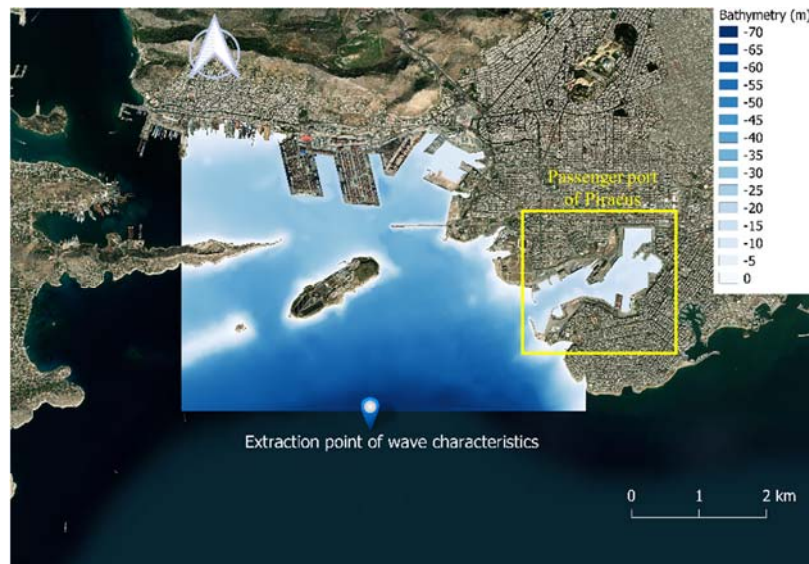
Figure 1. Passenger port of Piraeus, Greece, offshore wave data extraction point and computational bathymetry.
