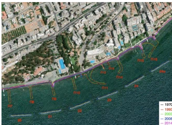
Figure 3 Satellite derived shoreline for Germasogia area in Limassol, southern Cyprus with shoreline positions over time indicated with different colors. Transect locations, E, F and G are indicated with white dashed lines (left to right) demonstrating a behaviour of -0.3\pm 0.1 , -2.1\pm 0.2 and -2.0\pm 0.3 m/yr, respectively
