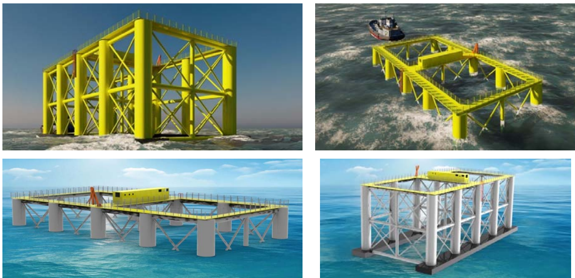
Figure 2. Animated design of the Open Sea semi-submersible fish cage structure for Cyprus
