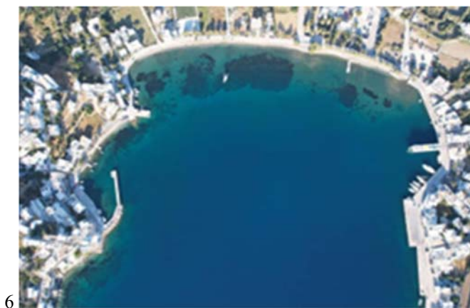
Photos 5 & 6. Satellite and drone photos of Katapola bay, before (5) and after (6) the construction of the fishing shelter (formed on the left side of Katapola bay's photo). The artificial pier's materials have been incorporated into shelter's breakwater and the beach has been already returned to its initial condition.
