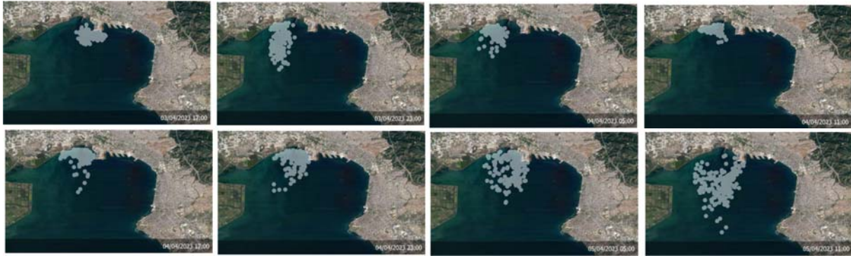
Figure 5 Snapshots of particles' spreading derived from the Wave4us forecast during an oil spill accident in the port of Thessaloniki (03/04/23)
