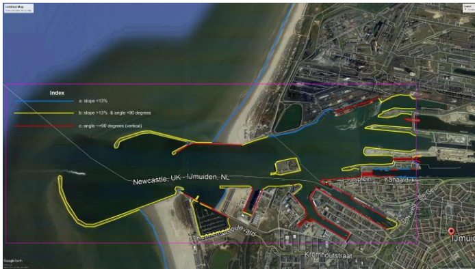
Fig. 3. Illustrative example map of reflection coefficient assignment on the perimeter of solid boundaries in Ijmuiden, NL, port 35 of Table 1, based on type of waterfront; a) natural beaches (blue color), b) absorbing jetties, rough armored slopes, and rubble mound breakwaters (yellow color), and c) fully reflective vertical quay walls (red color).
