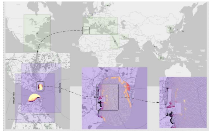
Fig. 2. Global chart depicting the locations of the selected 50 important ports of Table 1 (marked with purple dots). Green hatched areas correspond to model H domains. Zoomed windows refer to model A and B domains in the continental shelf and the port of Algeciras.
