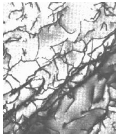
Fig.2.4a A transmission electron micrograph of titanium alloy in which the dark lines are dislocations [19].
