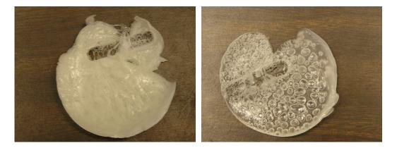
Figure 7.2 a) Composite of Surlyn and titania nanotubes.b) Surlyn prepared from neutralization of acid polymer using same procedure as the composite without the titania nanotubes
