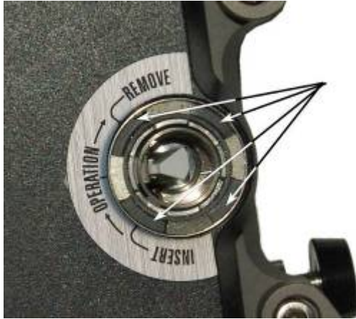
Fig. 1-5. Magnets for fixing the probe holder
