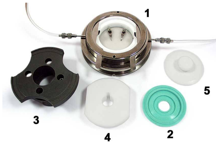
Fig. 2-2. Components of the liquid cell 1 – cell; 2 – diaphragm; 3 – cell holder; 4 – fitting tool; 5 – cover
