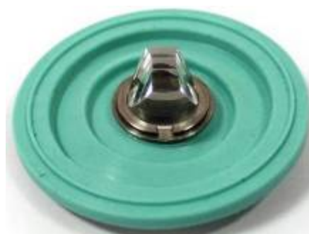
Fig. 4-3. Diaphragm fixed on the holder
