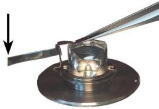
Fig. 3-1. Probe installation. The arrow shows the direction of force application
