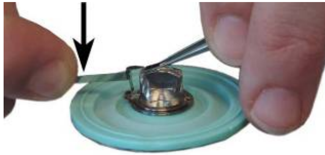
Fig. 4-6. Probe installation. The arrow shows the direction of force application
