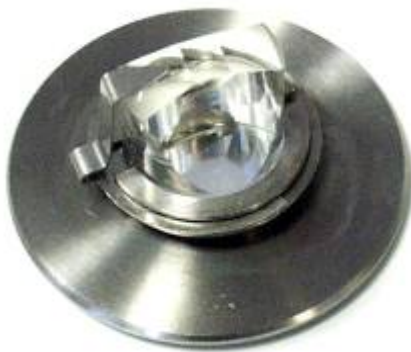
Fig. 1-7. Probe holder for operation in liquid
