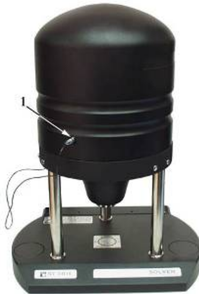
Fig. 6-1. The protective hood is installed on the approach unit 1 – grounding jack
