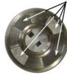
Fig. 1-6. Probe holder, view from below. The arrows show the location of the ferromagnetic sectors
