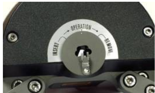
Fig. 1-15. Probe holder working position
