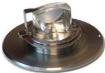
Fig. 1-3. Exchangeable probe holder for operation in liquid
