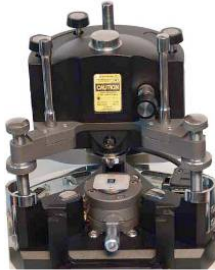
Fig. 3-13. The measuring head is installed in the approach unit
