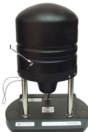
Fig. 2-22. The protective hood is installed on the approach unit 1 – grounding jack
