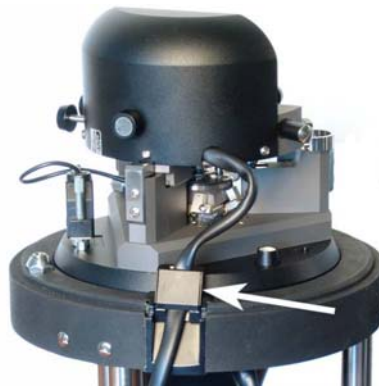
Fig. 2-21. The measuring head cable is secured in the holder
