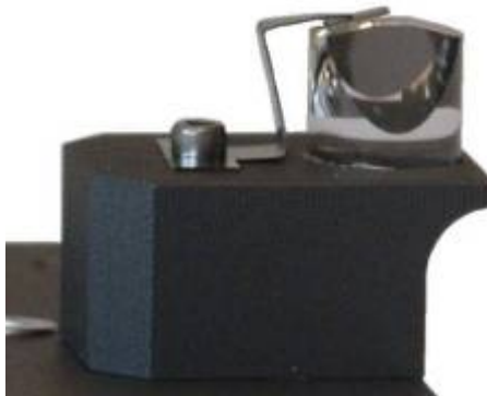
Fig. 2-2. Probe installed in the holder
