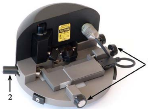
Fig. 2-4. Installation of the measuring insert on the measuring head 1 – XY screws for tuning the adjustment unit, 2 – hold-down
