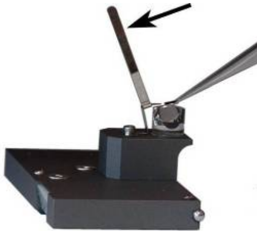
Fig. 2-1. Probe installation The arrow shows the direction of applied force
