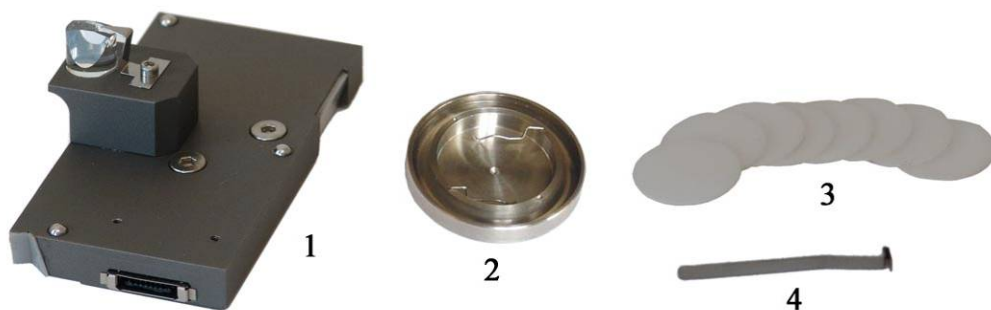
Fig. 1-2. Items included in the set of the measuring insert model AU028 with the open liquid cell
