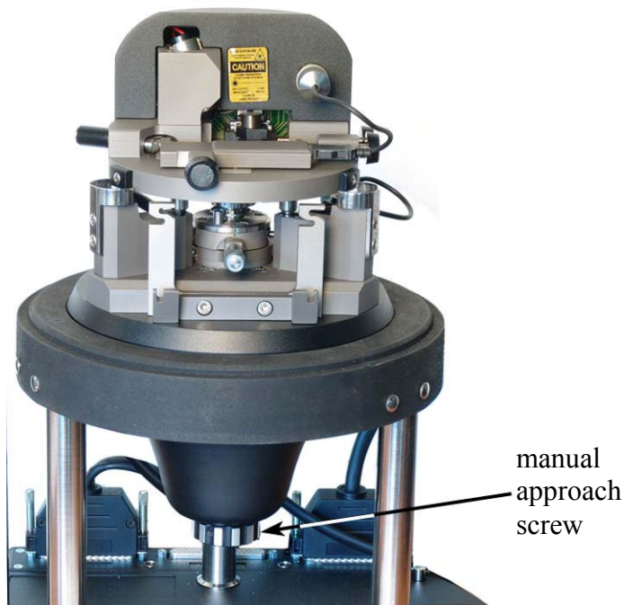
Fig. 2-12. Installation of the measuring head
