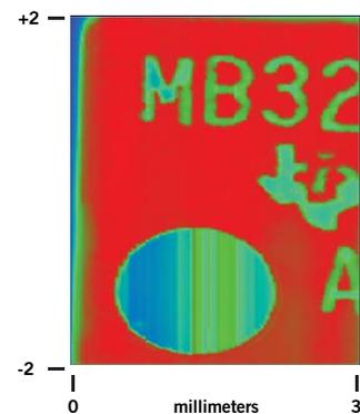
Figure 3. SECM area scan of same area of integrated circuit as figure 2 (SECM370).
