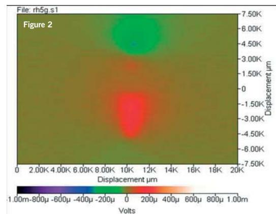
SVET image of region shown in figure 1, showing alternating anodic and cathodic behavior of the defect. The red region is cathodic behavior, and the blue is anodic.
