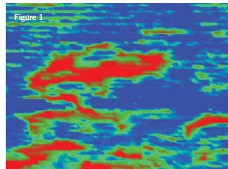
Figure 1. Polarized partially zinc-coated mild steel sample. Red areas show coating retained intact. (SDS370)
