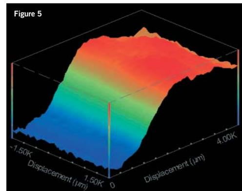
Scanning Kelvin Probe measurement over Indium Tin Oxide (ITO) / Organic LED interface
