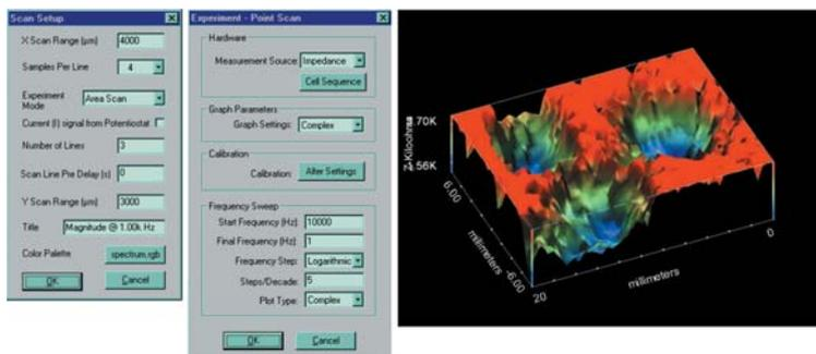
The LEIS370 software provides the user with a high degree of control over the experimental parameters as well as graphical features. The area scan images are easily exported into a text document as a bitmap image, or the data can be exported into a data spreadsheet for further analysis. The optional IsoPlot™ 3-D Surface Rendering Software allows the user to control viewing, light angles, color and plotting parameters.
