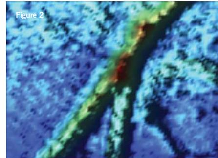
Figure 2. Open-circuit potential changes over zinc-coated sample due to scoring. (SDS370)
