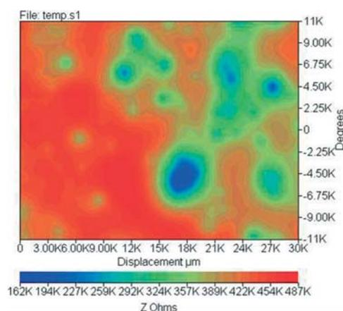
Localized impedance map of intact coating on mild steel with sub-film chloride contamination.
