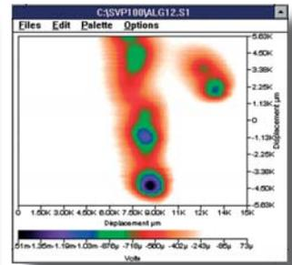
Time resolved SVET images representing current distribution associated with the development of corrosion activity in damaged coil coated steel. Images taken at one hour intervals.
