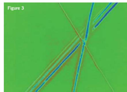
Figure 3. Optical surface profile of the scored zinc sample shown in figure 2. (OSP370)
