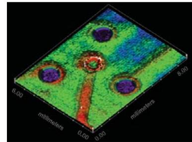
Figure 1. Non-contact surface profile of electrochemical sensor surface - sample courtesy of Oncoprobe Ltd.
