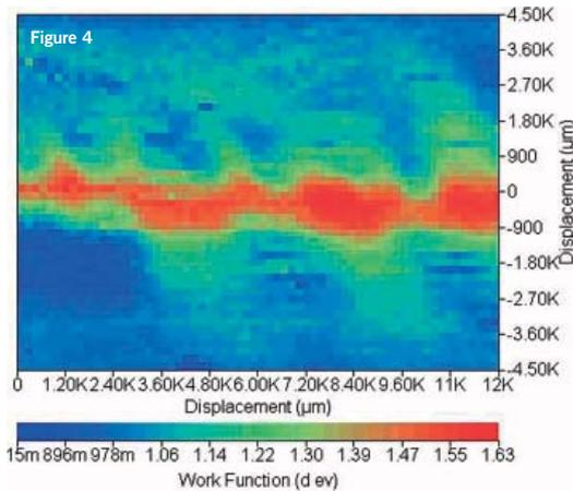
Scanning Kelvin Probe measurement of filiform corrosion on Aluminium.
