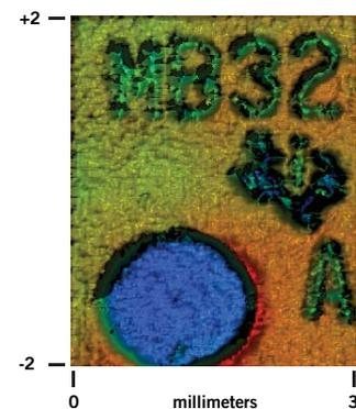
Figure 2. Non-contact surface profile of integrated circuit packaging (OSP370).
