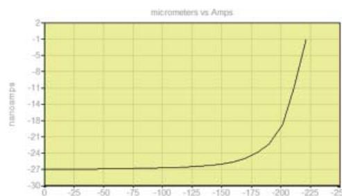
SECM approach curve to insulating surface for 10µm diameter probe.
