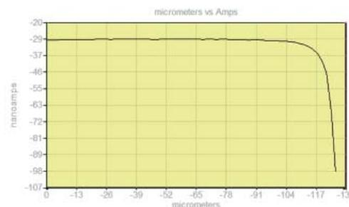
SECM approach curve to conducting surface for 10µm diameter probe.
