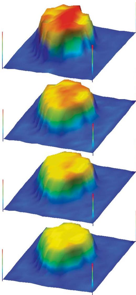
E<sub>corr</sub> changes due to flow rate variation on mild steel sample.
