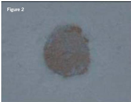
Optical image of an area of etched zinc coated steel
