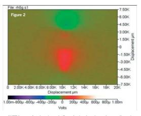
SVET image of region shown in figure1, showing alternating anodic and cathodic behavior of the defect. The red region is cathodic behavior, and the blue is anodic.
