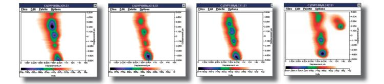
Time resolved SVET images representing current distribution associated with the development of corrosion activity in damaged coil coated steel. Images taken at one hour intervals.
