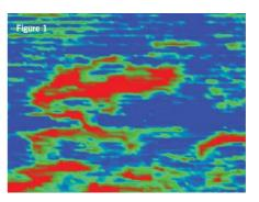
Figure 1. Polarized partially zinc-coated mild steel sample. Red areas show coating retained intact. (SDS370)
