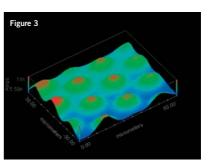
Isometric 3D projection of SECM image shown in figure 2. Peak current differences around 6nA.
