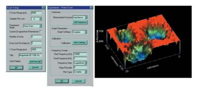
The LEIS370 software provides the user with a high degree of control over the experimental parameters as well as graphical features. The area scan images are easily exported into a text document as a bitmap image, or the data can be exported into a data spreadsheet for further analysis. The optional IsoPlot<sup>™</sup> 3-D Surface Rendering Software allows the user to control viewing, light angles, color and plotting parameters.
