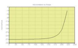
SECM approach curve to insulating surface for  $10 \mu m$  diameter probe.
