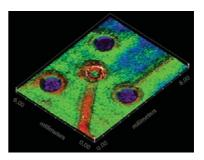
Figure 1. Non-contact surface profile of electrochemical sensor surface - sample courtesy of Oncoprobe Ltd.
