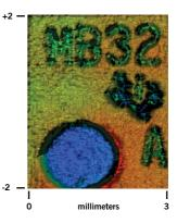
Figure 2. Non-contact surface profile of integrated circuit packaging (OSP370).
