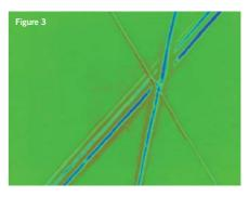
Figure 3. Optical surface profile of the scored zinc sample shown in figure 2. (OSP370)
