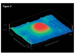
Surface map of Scanning Kelvin Probe signal recorded over area of sample shown in Figure 2.
