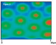
SECM image in tip-generation/substrate-collection mode of area shown in figure 1.
