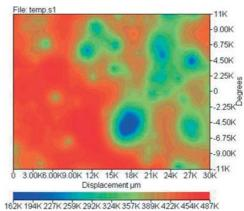
Z Ohms Localized impedance map of intact coating on mild steel with
