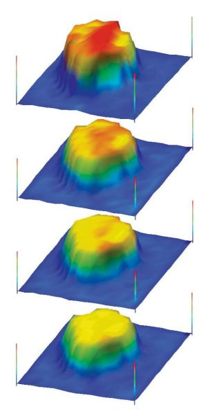
Ecorr changes due to flow rate variation on mild steel sample.
