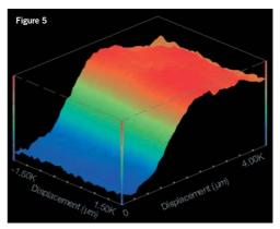
Scanning Kelvin Probe measurement over Indium Tin Oxide (ITO) / Organic LED interface
