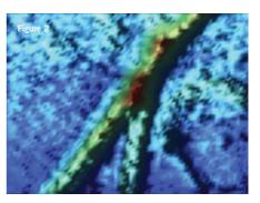
Figure 2. Open-circuit potential changes over zinc-coated sample due to scoring. (SDS370)
