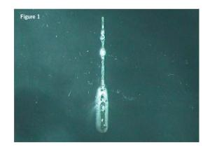
Optical micrograph of laser ablated, coil coated, galvanized steel.
