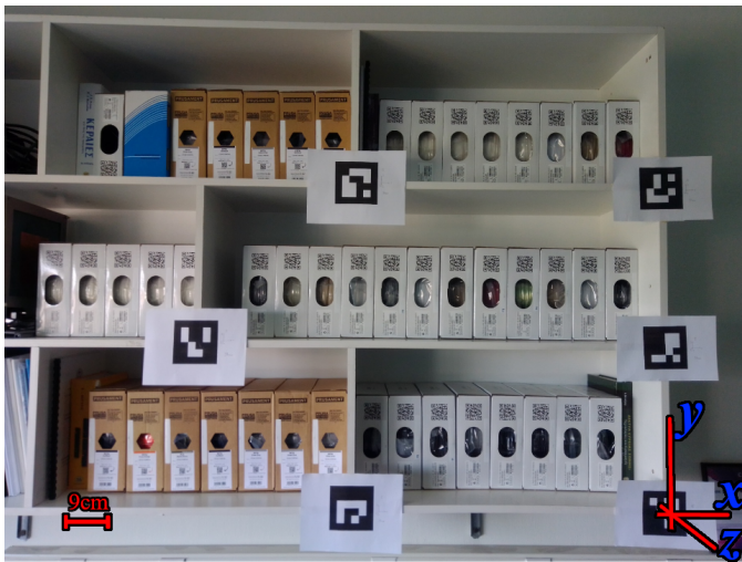
Fig. 12. RFID tagged optical landmarks were placed on the faces of some shelves. The handheld device was moved in front of the shelves, facing the landmarks. The trajectory of its antenna was calculated as explained in sections II-A to II-D, and was used, in order to calculate their positions.
