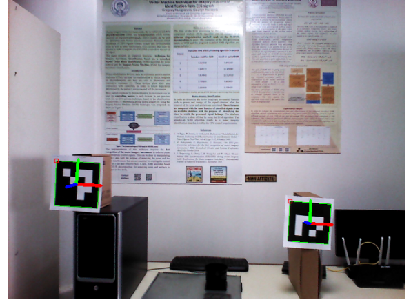
Fig. 4. An example of the detection of optical markers. The corners of the black squares are detected, and by the combination of the black and white blocks inside the square the orientation of the marker is extracted, as well as its id. The local coordinate system of each detected marker is also drawn on the captured frame.
