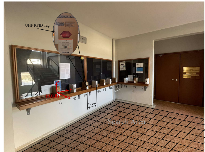
Fig. 18. The setup of the experiments with the portable reader.
