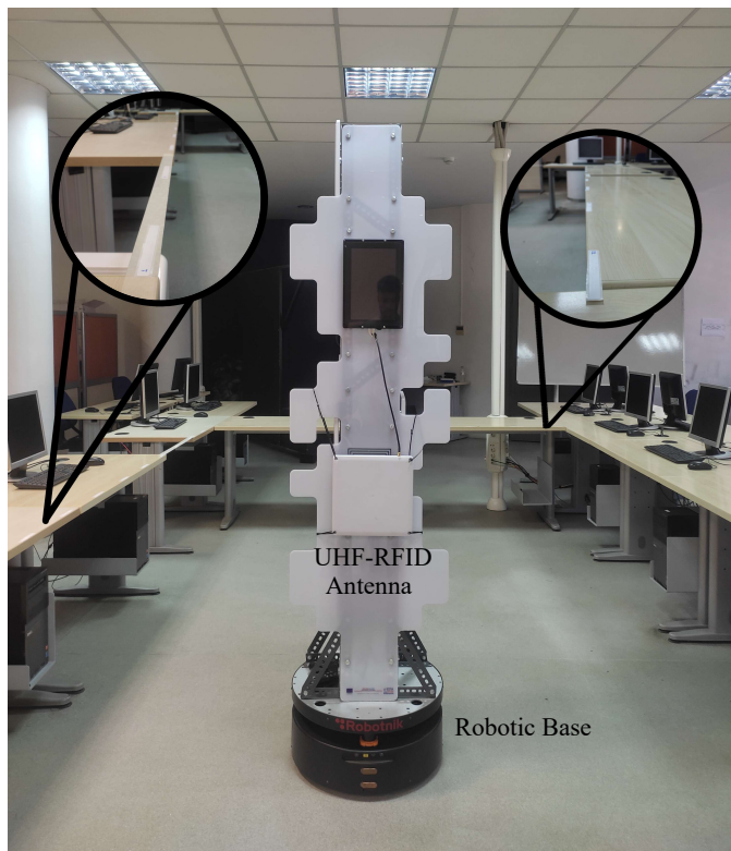
Fig. 12. The experiments' set up includes 22 tags, placed at a \Gamma configuration on top of desks in a multipath rich lab.
