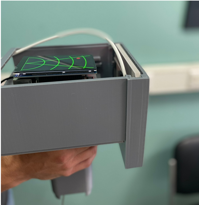
Fig. 1. Photograph of a prototype of the proposed device. The device is held so that the antenna is pointing in front of the user, and performs a "scanning" movement, as explained in section II. The target estimation appears as a red dot on the device's display, where the distance and the direction to it are indicated.
