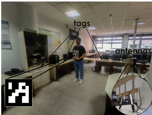
Fig. 11. Photo of the experimental set-up, where 4 antennas were employed opposite to 25 passive tags. The human target moves across the enclosed space carrying an ArUco marker such that the ground truth of its trace is measured.
