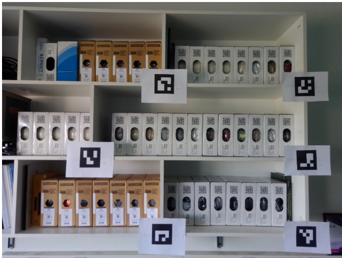
Fig. 4. Photograph of the experiment setup. Optical markers were placed on the faces of some shelves, and on top of them RFID-tagged items. The handheld device was moved in front of the shelves, facing the optical markers.
