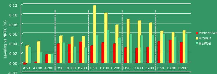
Fig. 2. Differences between the NRTK/MAC-derived heights (for station occupancies of 50/100/200 sec) and the spirit-leveled heights from R.
