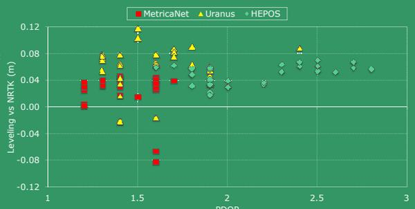
Fig. 4. PDOP-dependency of the differences between the NRTK-derived heights and the spirit-leveled heights as obtained in our tests at the five measured points.
