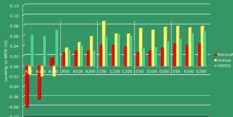
Fig. 3. Differences between the NRTK/VRS-derived heights (for station occupancies of 50/100/200 sec) and the spirit-leveled heights from R.
