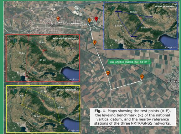
Fig. 1. Maps showing the test points (A-E), the leveling benchmark (R) of the national vertical datum, and the nearby reference stations of the three NRTK/GNSS networks.
