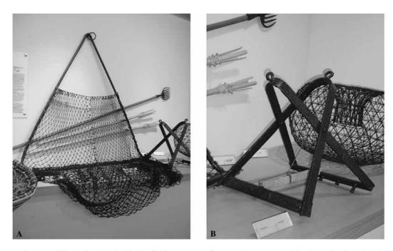
FIG. 2. Traditional dredges for bivalve fishing: A. "argalios" or "lagamna" used for the collection of scallops in the Gulf of Kalloni, island of Lesvos, North Aegean. B. "pinologio" used for the collection of fan mussels in the Greek Seas. Photos were taken at the Museum of Traditional Fisheries and Shells in Moudania (Chalkidiki, Greece) by D. Koutsoubas.
