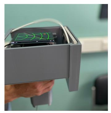
Fig. 1. Photograph of a prototype of the proposed device. The device is held so that the antenna is pointing in front of the user, and performs a "scanning" movement, as explained in section II. The target estimation appears as a red dot on the device's display, where the distance and the direction to it are indicated.
