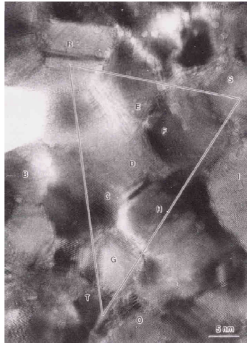
10 nm Au: 6-15 degrees relative grain rotation
