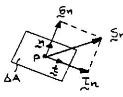
$$\begin{aligned}\tilde{S}_n &= S_n + T_n = S_n \cdot \tilde{\gamma} + T_n \cdot \tilde{\zeta} \\ S_n &= \lim_{\Delta A \rightarrow 0} \frac{\Delta F_n}{\Delta A}, \quad T_n = \lim_{\Delta A \rightarrow 0} \frac{\Delta F_t}{\Delta A} \\ \Delta F &= \Delta F_n \cdot \tilde{\gamma} + \Delta F_t \cdot \tilde{\zeta}\end{aligned}$$
