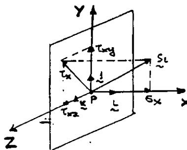
$$\tilde{S}_i = S_x \cdot \tilde{\gamma}_1 + T_{xy} \cdot \tilde{\gamma}_2 + T_{xz} \cdot \tilde{\gamma}_3$$
