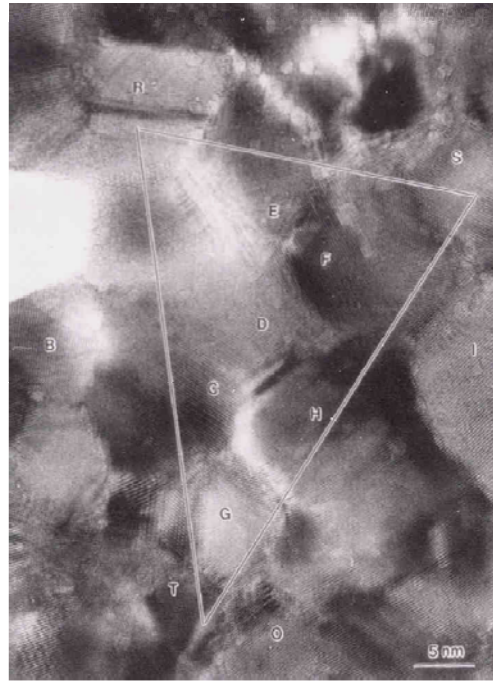
10 nm Au: 6-15 degrees relative grain rotation
