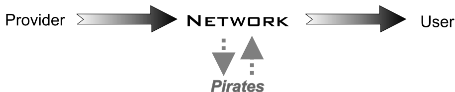
Figure 2: The elementary distribution system of digital products. Piracy for copyright violation or malicious modifications and retransmissions is possible.
