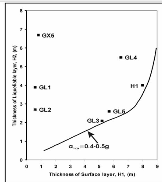
**Figure 6a.** Boundary curve proposed by Ishihara, 1985 for the effect of thickness of unliquefiable surface layer for surface disruption in the town of Lefkas
