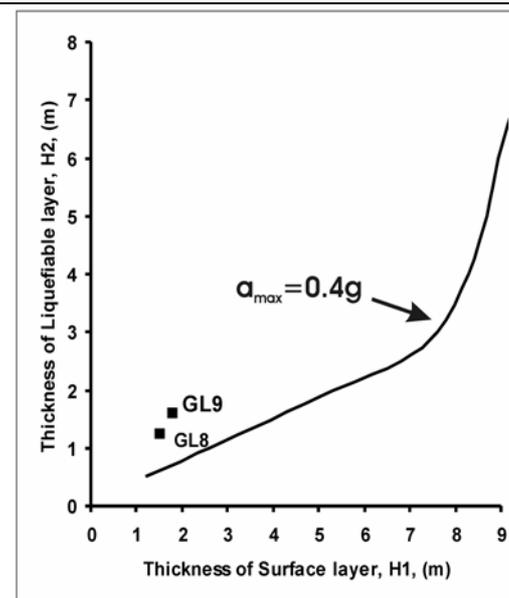
**Figure 6b.** Boundary curve proposed by Ishihara, 1985 for the effect of thickness of unliquefiable surface layer for surface disruption in the village of Lygia (GL8, GL9)
