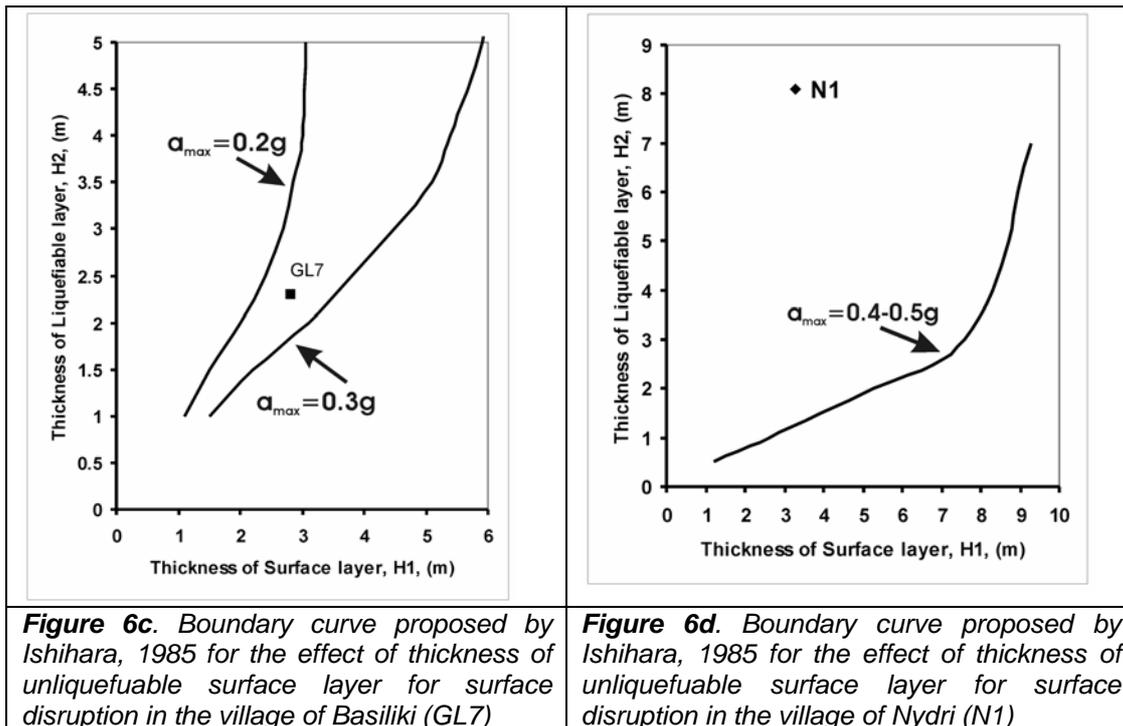
**Figure 6c.** Boundary curve proposed by Ishihara, 1985 for the effect of thickness of unliquefiable surface layer for surface disruption in the village of Basiliki (GL7)
