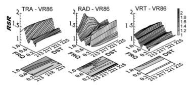
Figure 50. Russe site, Vrancea 1986 earthquake. Site amplification defined as RSR along the considered profile, mapped versus epicentral distance and frequency. Transverse (TRA), radial (RAD) and vertical (VRT) component are shown.
