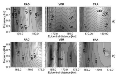
Figure 9. RSR versus frequency and epicentral distance for  $S_1$  (a) and  $S_2$  (b) profiles (Figure 8) in the case of May 30, 1990, displayed separately for the radial component (RAD), for the vertical component (VER) and for the transverse one (TRA).
