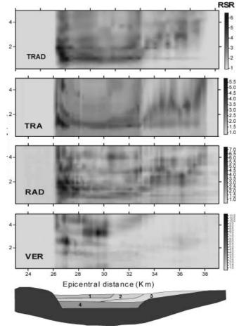
Figure 31. The cross section and the corresponding RSR versus frequency for VER, RAD and TRA. TRAD is the response spectra ratio assuming an epicentral distance of 150 km.
