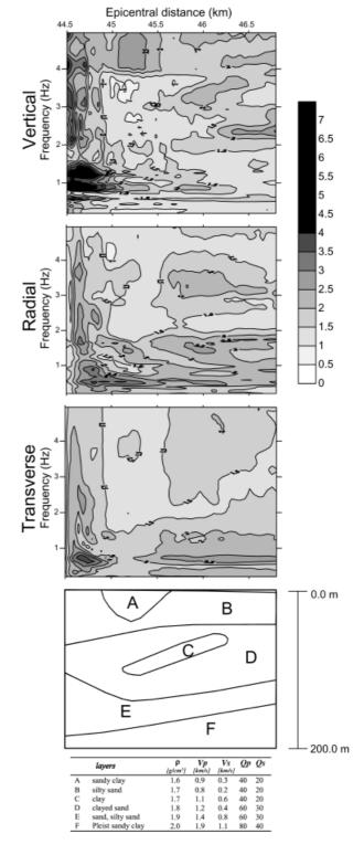
Figure 7. RSR (5% damping) versus frequency (Epicenter Gálospetri).
