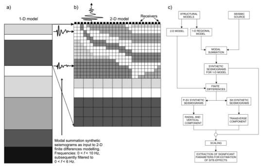
Figure 1. Schematic representation of the hybrid technique. The modal summation is applied considering stack of horizontal layers, each the bedrock model (a) to compute the input signals for the laterally varying part (b) where signals are of which is characterized by the propagated by finite differences numerical modeling to a set of sites on the surface. (c) Flow chart of the longitudinal and transversal algorithm.
