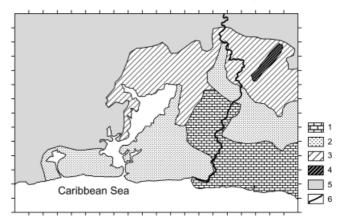
Figure 34a. Microzoning of Santiago de Cuba basin: 1-low RSR level, 2-intermediate RSR level, 3-high RSR level, 4-subzone of zone 3, where resonance effect was identified, 5-zone of El Cobre formation, not included in the analysis, 6-San Juan river; the ticks on the frame of the figure are 1km apart, the lower left corner has coordinates 19.945°N and 75.945°W.level.
