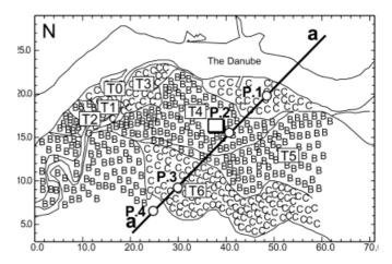
Figure 46. Scheme of the soil conditions at the site of Russe according to EUROCODE 8 crossed by the investigated profile a-a.
