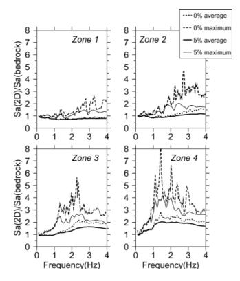
Figure 23. Maximum and average RSR for the four zones (for 0% and 5% damping).
