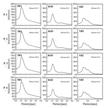
Figure 49. Russe site, Vrancea 1986 earthquake. Response spectra for 5% damping, SA  $(cm/s^2)$ , at receivers P.1, P.2, P.3 and P.4 located along the profile a-a, shown in Figure 46. Transverse (TRA), radial (RAD) and vertical (VRT) component are shown.
