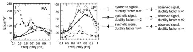
Figure 48. Validation of the theoretical results considering the recorded accelerations at Russe due to the Vrancea 1986 earthquake. Absolute energy input (Uang and Bertero, 1990; Decanini and Mollaioli, 1998) for three ductility factors for East-West (EW) and for the vertical (UP) components for both theoretical (solid line) and observed (dashed line) signals are shown.
