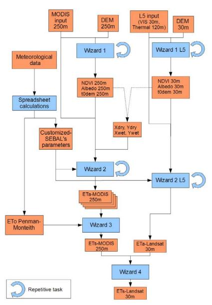
Figure 4. Operation scheme of the ITA-Water tool.
