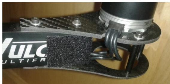
Figure 3. Cables were not in contact with the metal parts after modification
