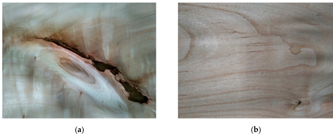
Figure 3. Poplar wood sliced plain-cut veneer sheet with live knot and decay (a), and cherry wood veneer with irregularities of annual rings (b).
