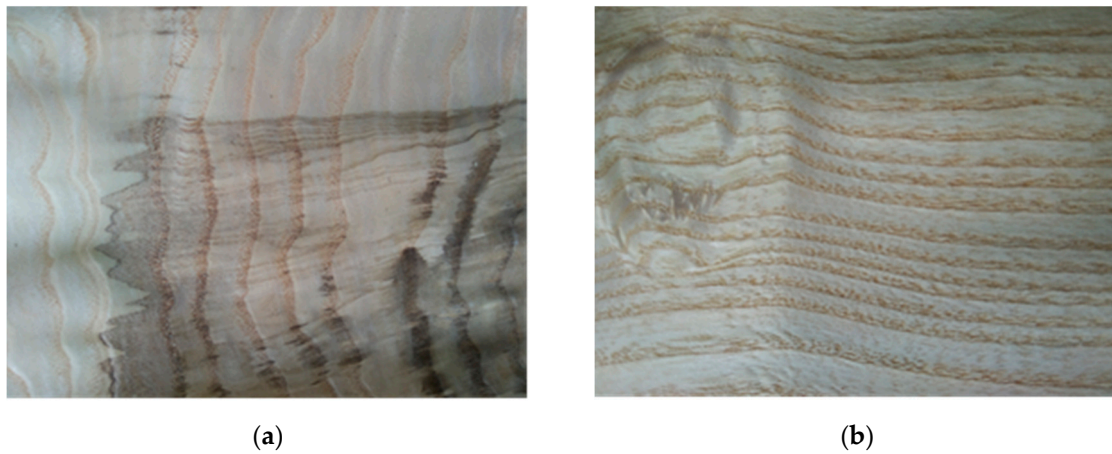
Figure 2. Ash wood sliced veneer with discoloration and irregularities of annual rings (a), and live internal knot with spiral grain around the knot (b).
