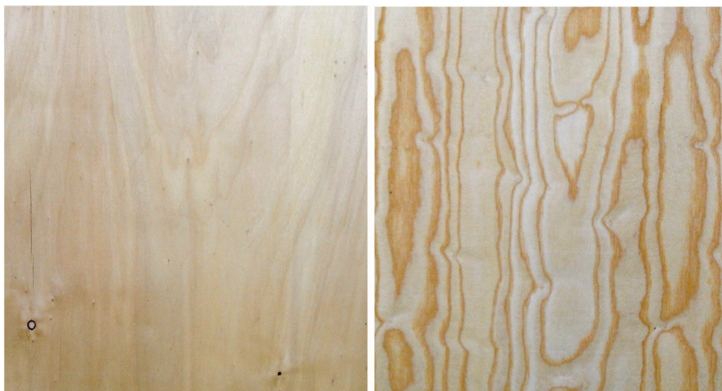
Photo 1. Surface appearance of the two 3-ply plywood studied (Poplar – left, Tree-of-Heaven – right).
