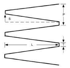
Fig. 1 Design variables of a finger-joint: Pitch (P), Length (L), Slope (S), and Width of fingertip (T).
