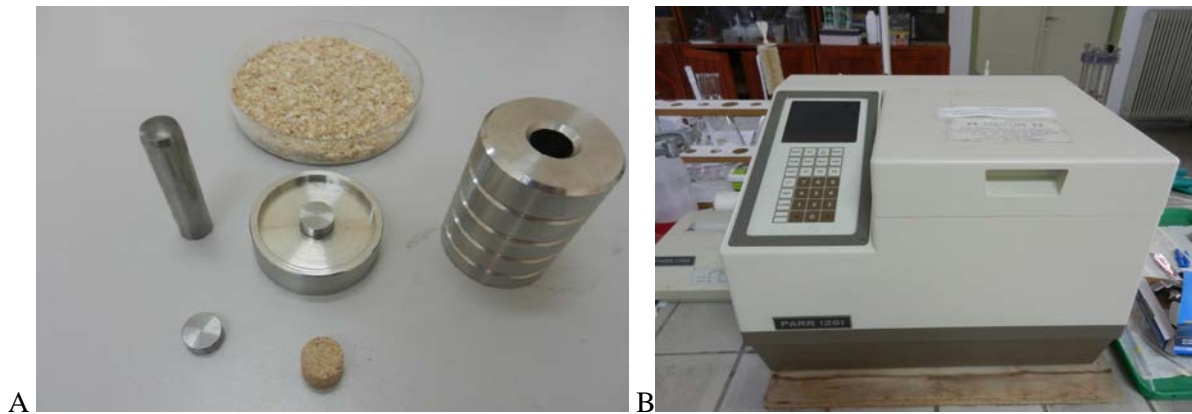
Figure 2 A. Pellet press with its accessories, B. Parr 1261 isoperibol bomb calorimeter
