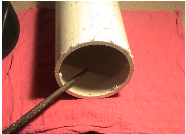
File off the sharp burrs and edges
