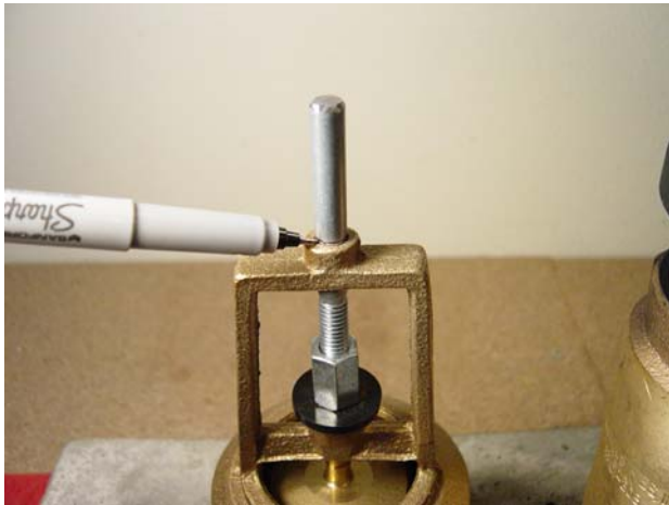
Marking the travel limits
