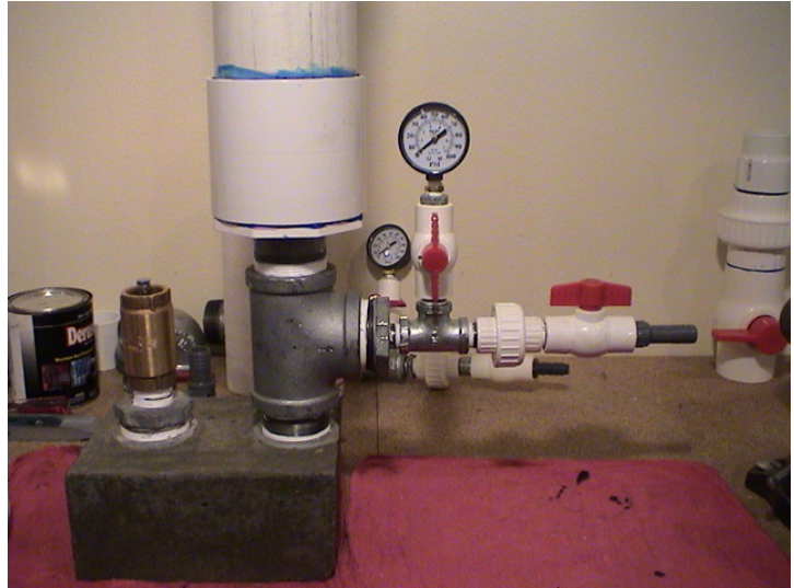
Adding ball valves, gauge and union
