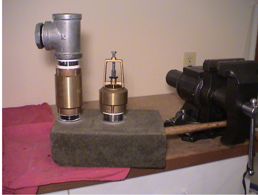
Using a 2lb Hammer Handle in the vise for added leverage.
