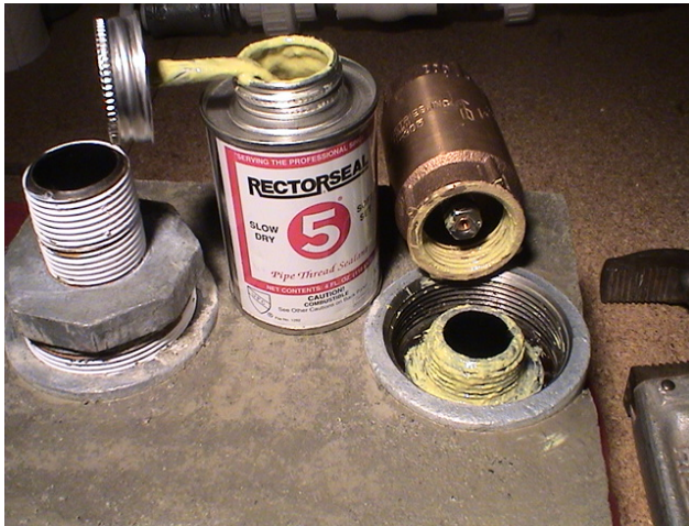
Applying liquid thread sealant
