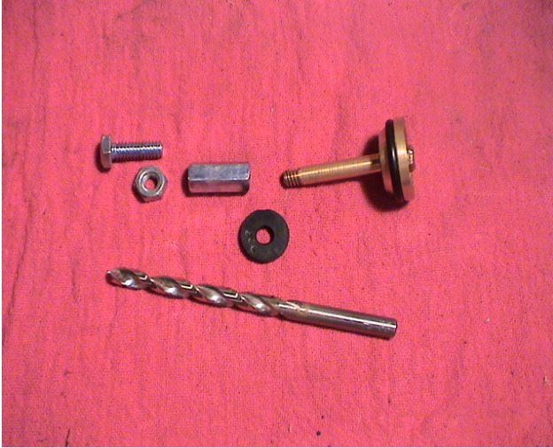
Waste / Impetus Valve Conversion Parts
