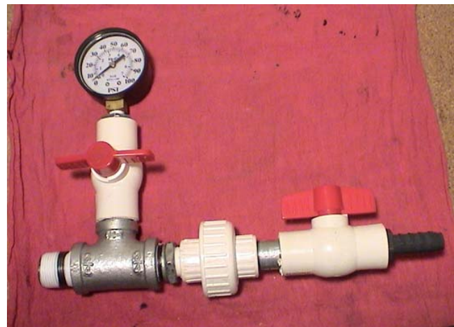
Completed Valve / Gauge Assembly
