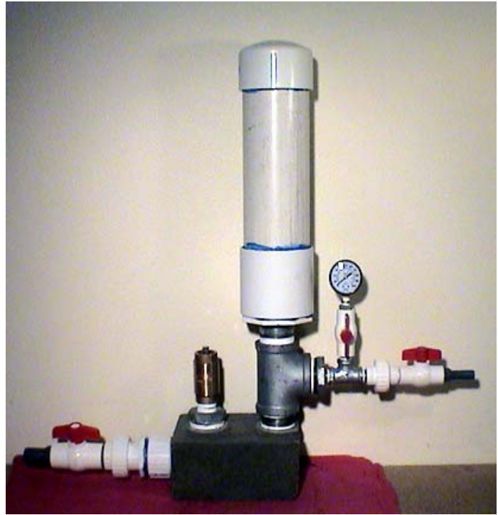
Completed HRP1-1 Pump ready to paint
