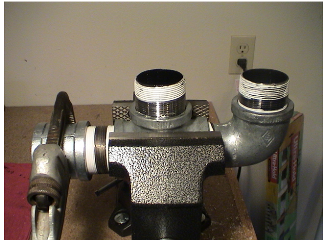
Adding the 2" Coupler after painting inside
