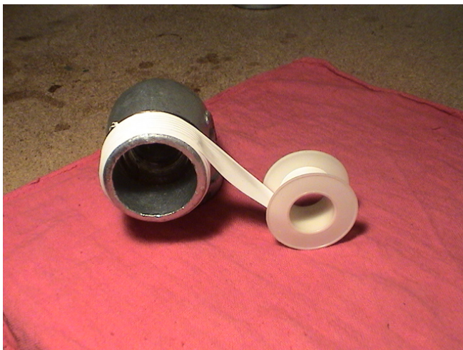
Wrap the Teflon tape clockwise
