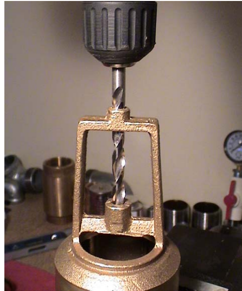
Drilling out to fit the 5/16" hardware
