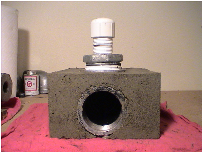
HRP1-1 after removing forms
