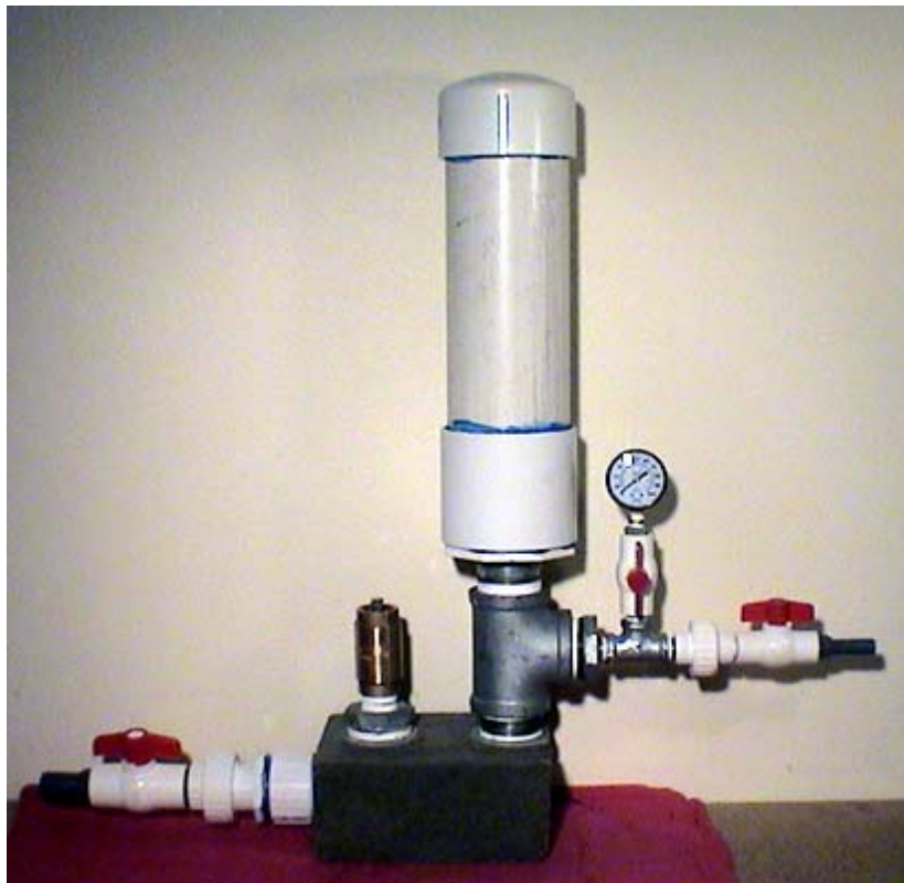
HRP1-1 Completed Pump
