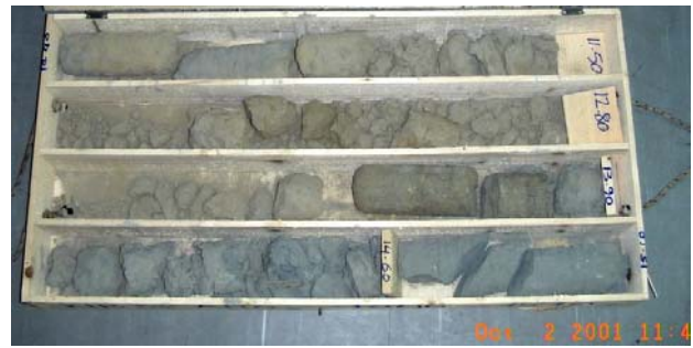
Figure 3. Bore Hole samples from Olympia (sound marl: deeper than 13.80 m)
