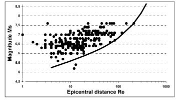
Figure 2. Magnitude versus epicentral distance (Re). With circles are the data and the solid line is the critical line proposed at the present paper.
