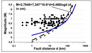
Figure 4. Magnitude versus Fault distance (Rf). With circles are the data and the solid line (blue) is the critical line proposed in the present paper. The dashed lines (1) and (2) are the curves proposed by Ambraseys and Papadopoulos & Lefkopoulos.
