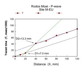
Figure 4. Ultrasonic velocities measured on the surface of calcarenite blocks, treated with consolidation liquid. The change of the regression slope corresponds to both consolidation and weathering depths.
