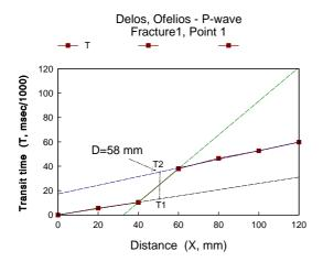
Figure 8. Ultrasonic velocities diagram on the surface of Ophelios marble statue (Delos island, Greece), for estimating the depth of a crack along its left leg.
