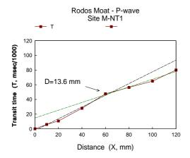
Figure 3. Ultrasonic velocities measured on untreated surface of calcarenitic blocks. The change of the regression slope corresponds to the depth of the weathered zone.
