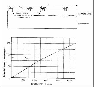
Figure 2. Diagram showing the depth of the damaged  $layer(PUNDIT Manual^{5})$
