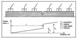
Figure 7. Diagram showing the depth of a crack, on the surface of a stone (PUNDIT Manual<sup>5</sup>)
