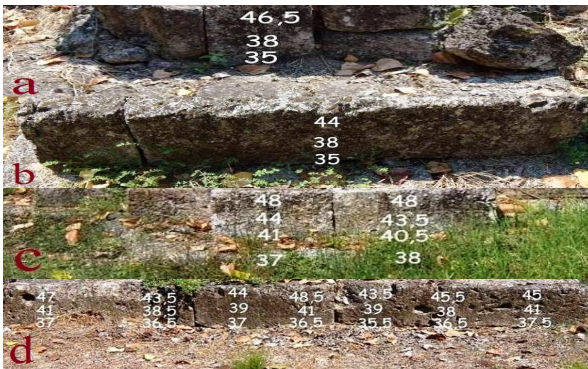
Fig. 3 IR thermometer measurements, sunny conditions, Asklepios temple, a) north side, b) east side, c) south side, d) west side
