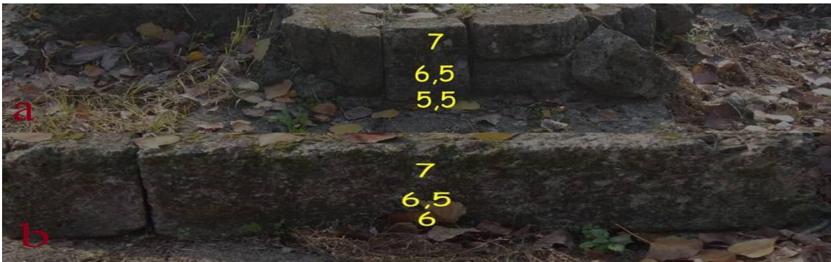
Fig. 5 IR thermometer measurements, wet conditions, Asklepios temple, a) north side, b) east side, c) south side, d) west side
