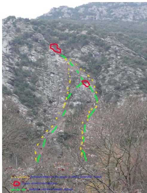
Figure 3. Fall track of the boulders (red circles indicate the source area and green lines show the path)
