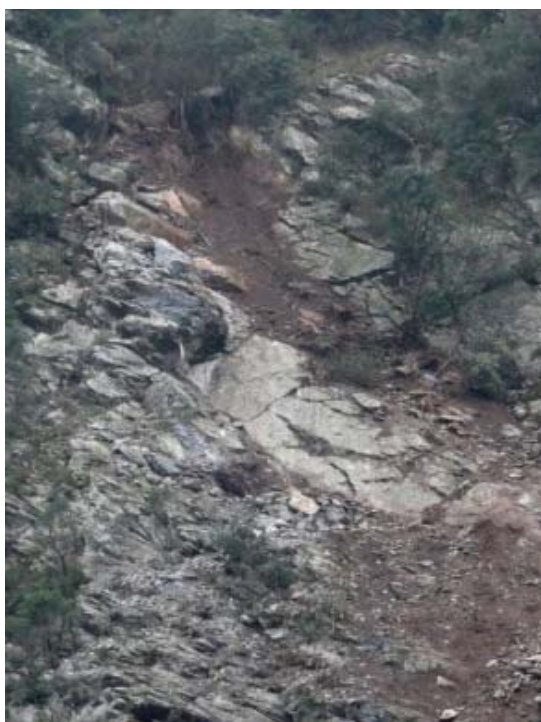
Figure 6. The initiation of the slope failure originated as sliding along the joint 350/47
