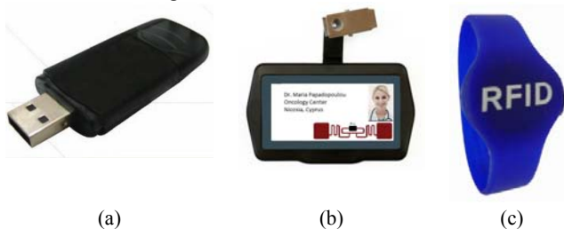
Fig. 2. (a) Stick-like USB/UHF RFID reader/writer; (b) RFID enabled plastic identification card; (c) RFID wristband.
