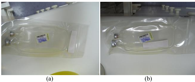
Fig. 21. RFID tag placed: (a) on the plastic edge of the bag; (b) in the middle of the bag (liquid underneath).
