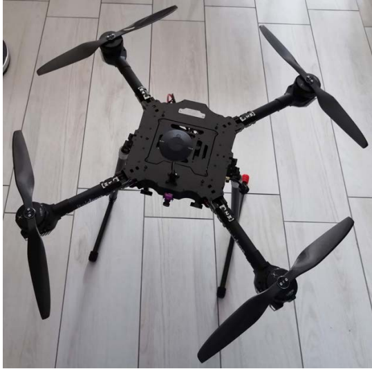
Fig. 2. Prototype drone for UHF RFID inventorying.
