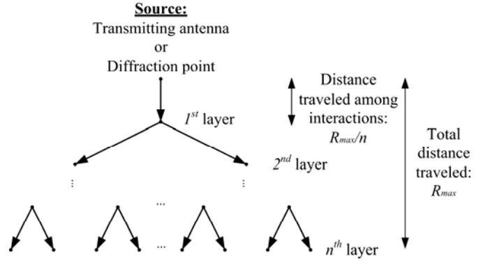
Fig. 9. Ray splitting after successive incidences.
