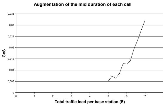
**Figure 6.** Variation of GoS dependent on the total traffic per base station
