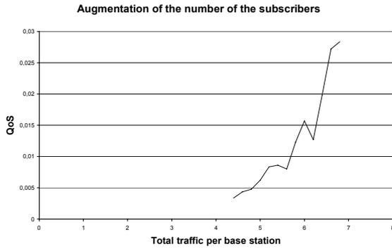
**Figure 5.** Variation of QoS dependent on the total traffic per base station.
