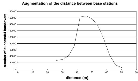
**Figure 4.** Variation of the number of successful handovers while incrementing the distance between base stations.
