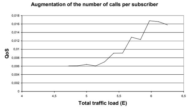
**Figure 7.** Variation of QoS dependent on the total traffic per base station.
