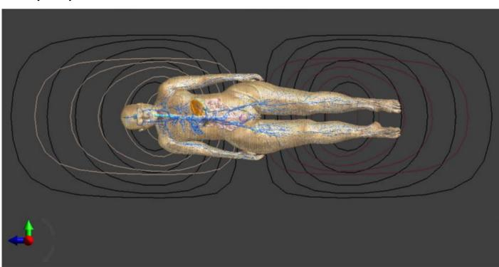
Continuous lines around the human body represent the gradient field lines
