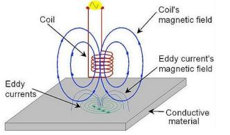
AMF generator system produces not only a magnetic field, but also an electric field. The electric field penetrates normal tissue and induces eddy currents, which result in unwanted heating of normal tissues.
